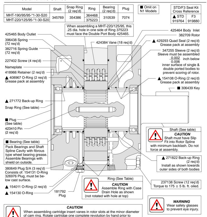
assembly with bodies to prevent misalignment of springs and guides.
