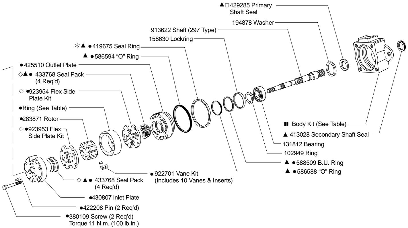
6 SAE rated capacity (45\*\*VQ shaft end cartridge)
