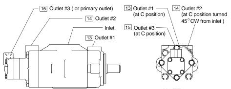
**NOTE**V10 cover can be assembled in any of four positions refer to drawing M–2005–S.
