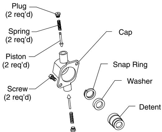
**Detent used on "C" Float Section**
