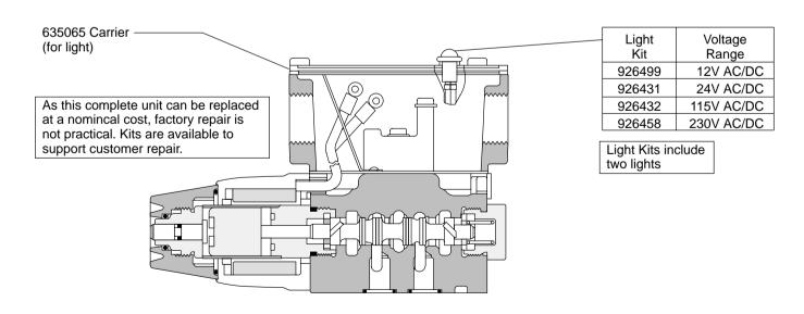
For satisfactory service life of these components in industrial applications, use full flow filtration to provide fluid which meets ISO cleanliness code 20/18/15 or cleaner. Selections from Eaton OFP, OFR, and OFRS series are recommended.
