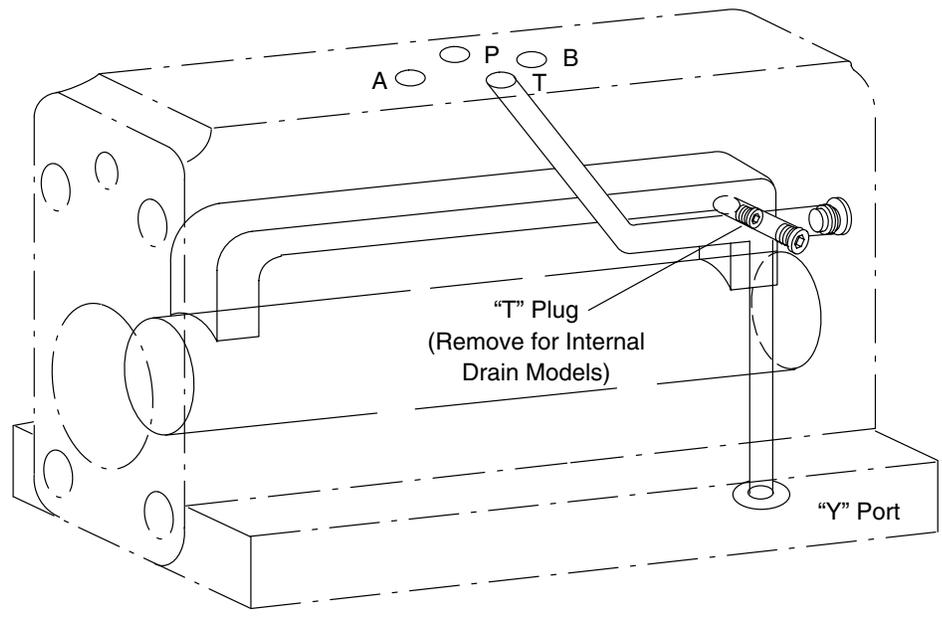
Figure 23c. DG5S4-04-T-40 Internal Pressure Passages & Plug Locations
