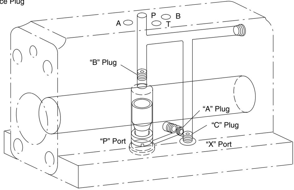
Figure 23b. DG5S4-04-(K/R/S)-40 Internal Pressure Passages & Plug Locations
