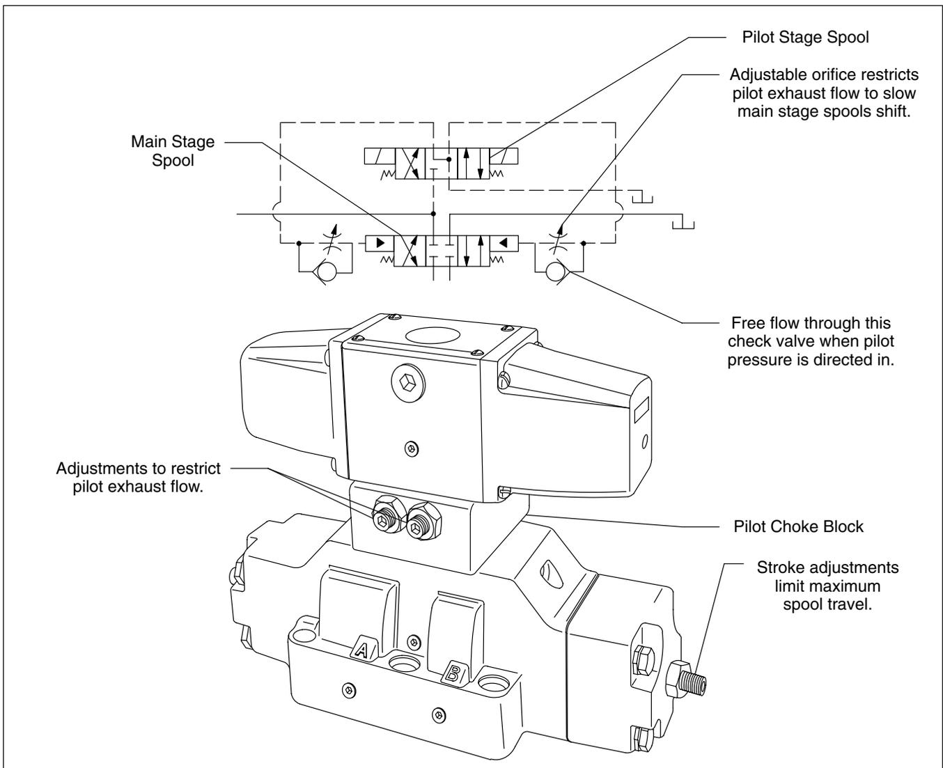
Figure 10c. DG5S4 with Pilot Choke & Stroke Limiter Options
