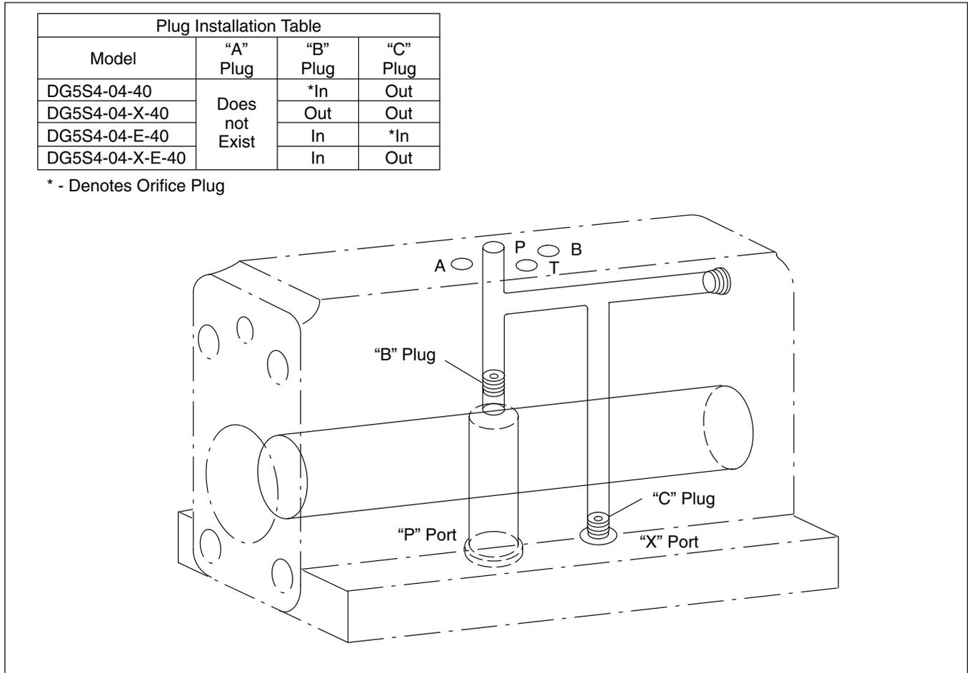
Figure 23a. DG5S4-04-X-40 Internal Pressure Passages & Plug Locations
