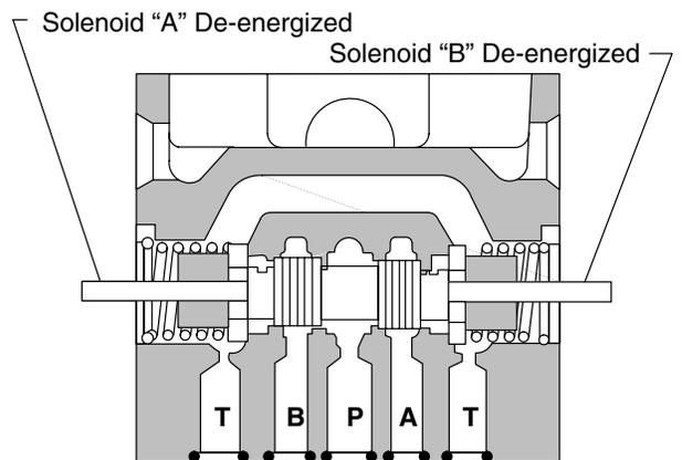
12c. Flow Conditions Blocked (Center Condition #2 Spool)
