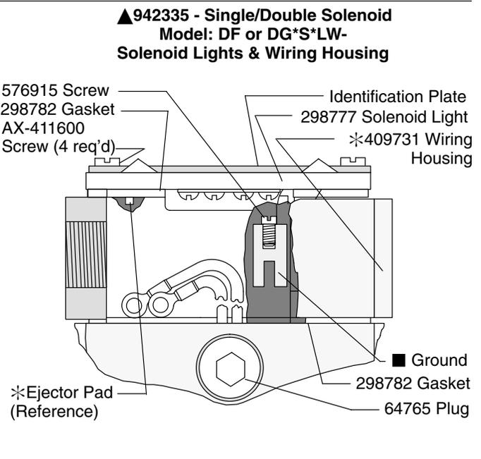
● Assemble with circuit breaker and light over solenoid.
