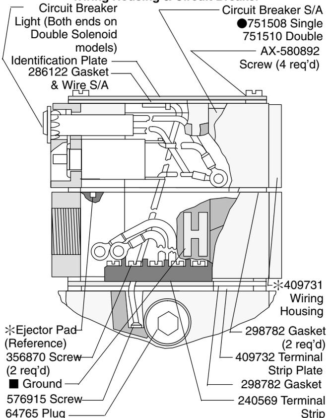
Assemble housing with ejector pads and with electrical conduit connection over solenoid "B". (Solenoids "A" and "B" are identified on units by diagram plate on side of pilot valve. For type "4" and "8" spools conduit connection location on end of "W" wiring housing is reversed).
