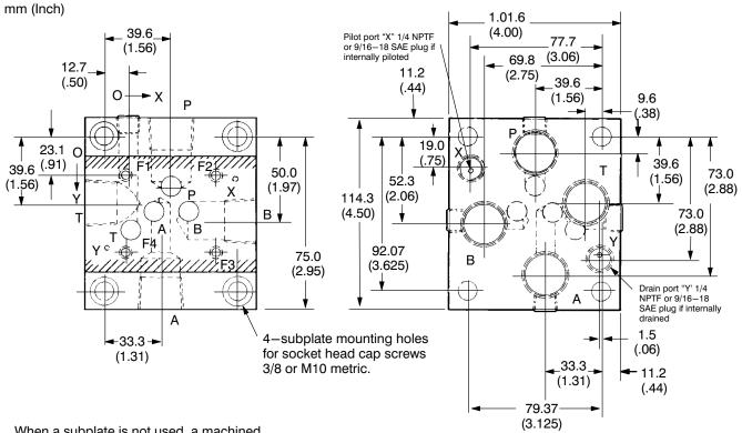
When a subplate is not used, a machined pad corresponding to the shaded area must be provided.
