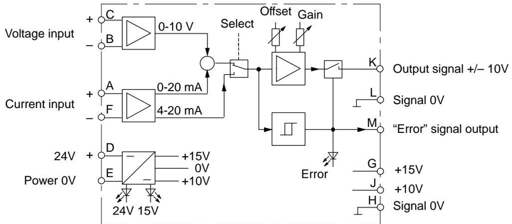
**Note:** The unused input signal pin B or C must be connected to signal 0V (pin H or pin L).
