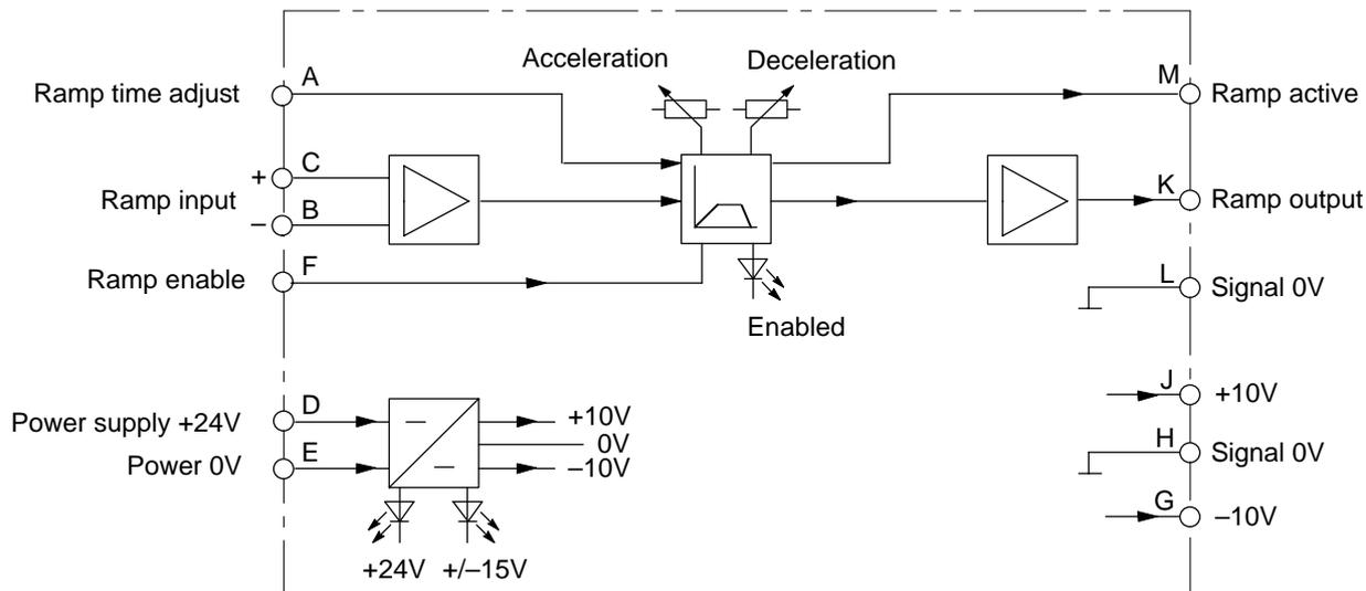
**Note:** The unused input signal pin B or C must be connected to signal 0V (pin H or pin L).
