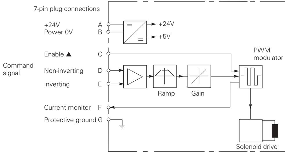
▲ In valves with PH7 or PR7 type electrical connection.
