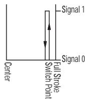
Signal 0 = Voltage at pin 4 = 0V
