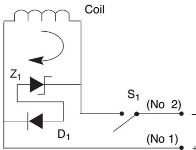
*NOTE: These surge suppression devices are "Polarity Dependent." Proper biasing conditions must be met when installing/connecting a coil in a system.*
