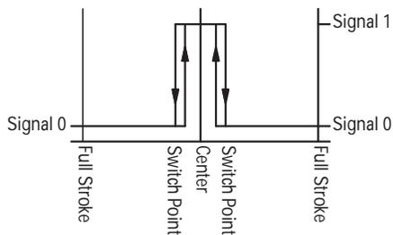
Signal 0 = Voltage at pin 2/4 < 1.8V
