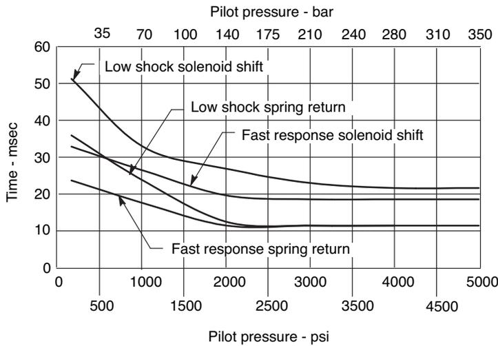
SPRING CENTERING TIMES @ RATED FLOW & PRESSURE
