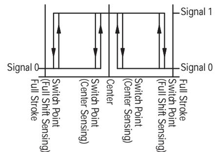
Signal 0 = Voltage at pin 2/4 < 1.8V
