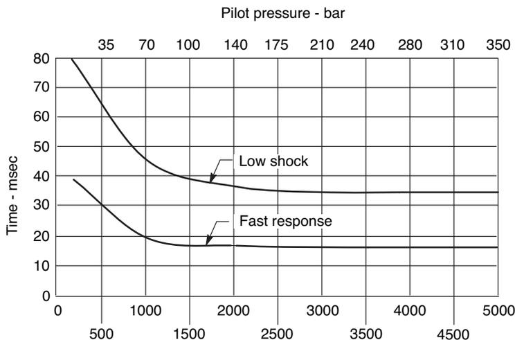
Centering Times for Pressure Centered Valves @ Rated Pressure (A to P or B to P)
