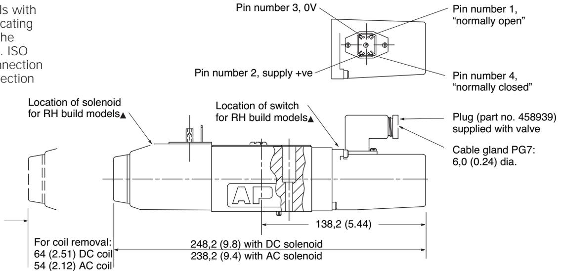
▲ For LH build (DG4V-3-\*AL) solenoid and switch locations are reversed.
