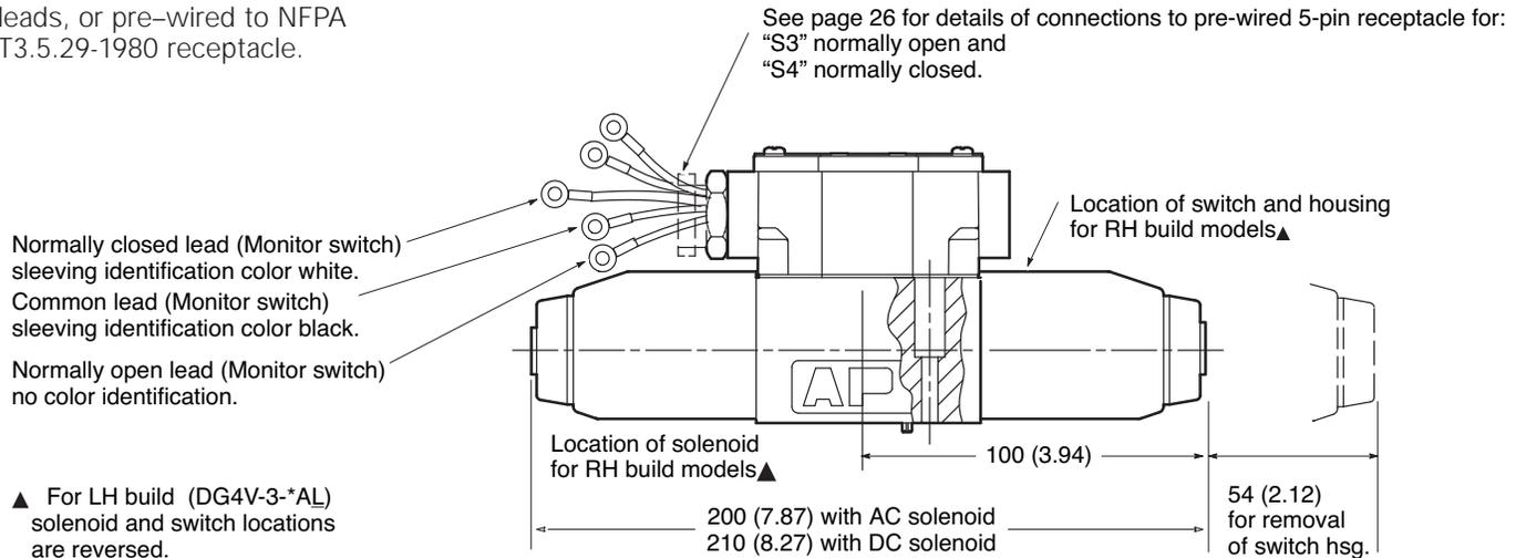
▲ For LH build (DG4V-3-\*AL) solenoid and switch locations are reversed.
