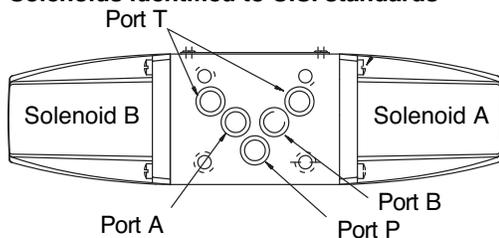
Functional symbols related to solenoid identity "A" and/or "B" according to NFPA/ANSI standards, i.e. energizing solenoid "A" gives flow P→A, solenoid "B" gives flow P→B (as applicable).
