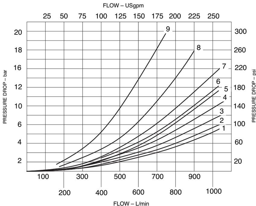
1. Figures in the pressure drop chart give approximate pressure drop ( $\Delta P$ ) when passing 473 l/min (125 USgpm) flow (Q) of 35 cSt (164 SUS) fluids(s) having .865 specific gravity.
