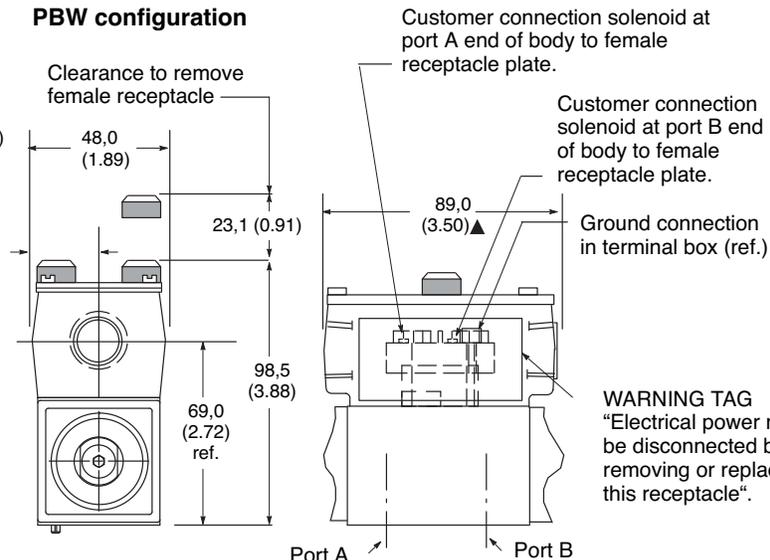
▲ The conduit box dimensions used for the PA/BBW type connector are different from those on the other "F" type coil models.
