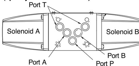
Functional symbols related to solenoid identity "A" and/or "B" according to European convention i.e. solenoid "A" adjacent to "A" port, solenoid "B" adjacent to "B" port of valve.
