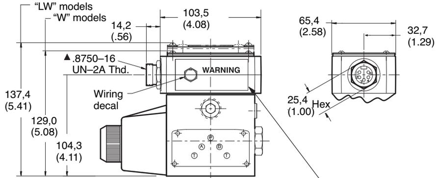
▲ Electrical connection is over solenoid on single solenoid models, and over "b" solenoid on dual solenoid models. See diagram plate for "b" solenoid location. Electrical rating 600 volts, 3 pole, 10 amps and 5 pole, 8 amps. The female portable plug to be furnished by customer.
