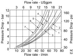
NOTE: For spool types 3 and 6; not recommended for flows in excess of 60 l/min (15.8 USgpm).
