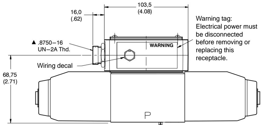
Warning tag: Electrical power must be disconnected before removing or replacing this receptacle.
