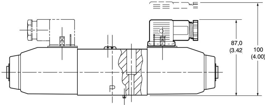
Connector can be positioned at 90° intervals on valve by re-assembling contact holder into appropriate position inside connector housing.
