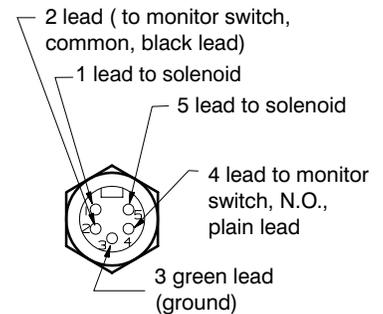
▲ Electrical connection is over solenoid on single solenoid models, and over "b" solenoid on dual solenoid models. See diagram plate for "b" solenoid location.
