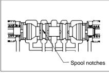
Spools with contoured or notched lands are used to provide maximum control of flow rate change as the spool is shifted.
