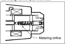
Spool shift speed is controlled by a metering orifice in the solenoid. Three orifice sizes are available to meet your application.
