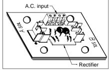
Conventional alternating current (120/60 or 110/50) input is converted to D.C. through a rectifier located in the terminal box.
