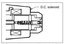
D.C. solenoids prevent coil burnout during controlled rate of solenoid shift.
