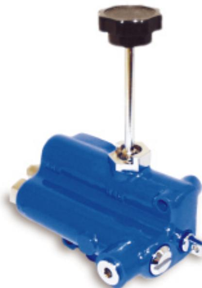
Similar to other single spool control valves, this valve allows the operator to smoothly position (raise and lower) the mower deck or reels with precision. In addition, lift circuit back pressure can be modulated by operating a rotary needle cartridge which allows the operator to take weight off the cutting units for reduced ground pressure and increased tractive effort or to apply down pressure to the cutting units for improved cutting finish.
