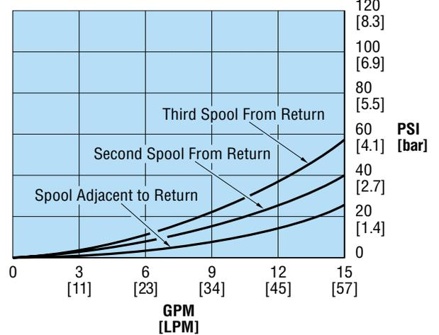
**Work Port Pressure Drop Flow: Inlet to Work Port**
