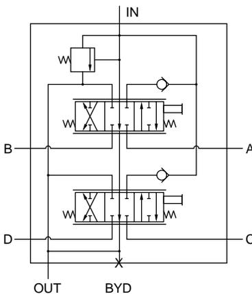
Note: Spool 3 is in tandem with spools 1 and 2; this allows metering to spools 1 and 2 with all excess flow to spool 3.
