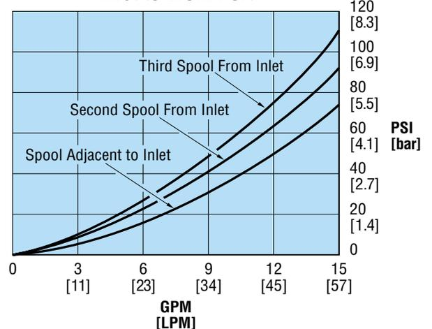
Tests performed with oil viscosity 150 SUS at 100° F [37.7° C] – oil temperature 130° F [54.4° C].
