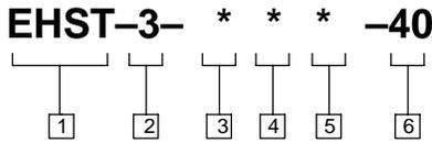
**1 Proportional Pressure Control with Integrated Electronics**
