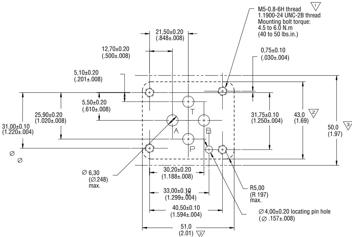
1 The minimum thread depth is 1.5 of bolt diameter. The recommended full thread depth is  $2xD+6\text{mm}$  to aid in the interchangeability of valves and to reduce the number of fixing bolt lengths. The recommended engagement of fixing bolt thread for ferrous mountings is 1.25 D.
