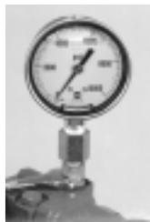
flow compensator pressure exceeds 15 bar [210 PSI]. Use a gauge that is dampened or glycerine filled. With the gauge installed and the load sensing valve in the closed position, start the system and observe the flow compensator pressure. If the reading is other than 13 to 15 bar [190 to 210 PSI], readjustment of the flow compensator may be required.
