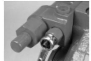
3) To change setting, remove the adjustment screw cover from the flow compensator valve. Loosen the flow compensator adjustment screw lock nut with a 7/16 inch open end wrench.
