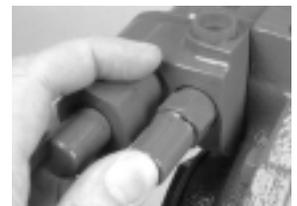
**To check or readjust pressure compensator valve setting:**
