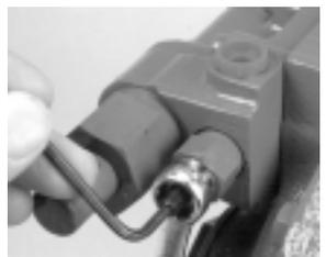
6) After turning system off, install the compensator screw cover and check pressure compensator settings.
