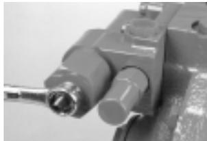
10) To readjust the pressure compensator you must first use a 7/16 inch open end wrench to loosen the compensator adjustment screw lock nut.
