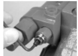
5) After adjustments are complete, hold the adjustment screw stationary and tighten the locknut to (torque 8 to 11 N•m [6 to 8 lbf•ft]).
